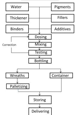
The figure shows the following working process during the production of internal paint systems: First, the silos and weighting containers are filled, followed by transportation and adjustment of raw material into the mixer for dispersion. After a quality control, the internal paints are filled into containers. Then they are loaded and delivered.
